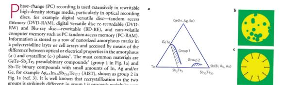
Figure 1 | Phase diagram of PC materials and crystallization patterns. **a**, The most commonly used materials for optical recording are in groups 1 and 2. **b**, Nucleation-dominated recrystallization (as in GST). **c**, Growth-dominated recrystallization (AIST).
